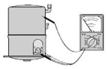
Figure 2: Typical ground test
